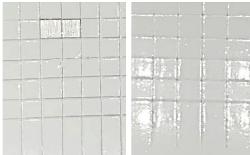
Aluminum Cold Rolled Steel 15 mil WFT, Cured 7 Days, Permacel Tape
