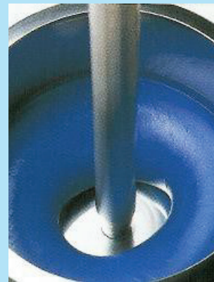
Figure 1 Mill base for a coating
