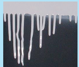
Figure 3b Waterborne emulsion coating with 'runners'
