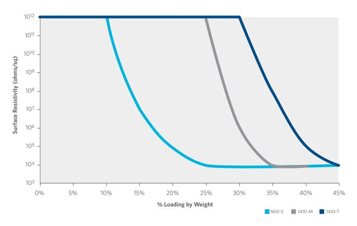
This example illustrates the ability to control the desired surface resistivity in epoxy resin by Zelec® ECP selection and loading.
